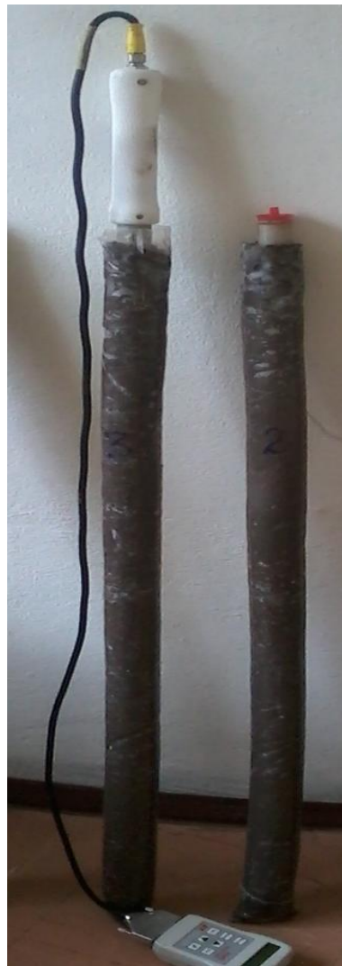
Figure 3.5: PR2/6 and PR2/4 soil moisture profile probe and working principle; Source: User Manual, Delta-T Devices, 2004 (left), PR2/6 calibration process under controlled soil moisture content (right)
